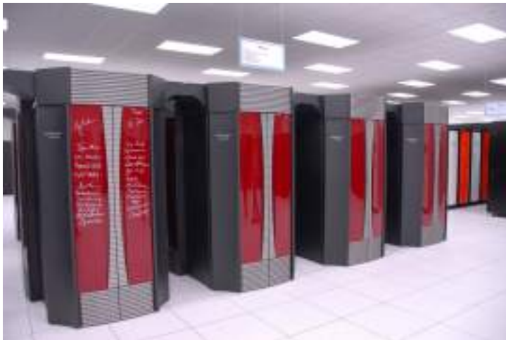
Cray X1 (2005, 15 million dollars, 166,4 Tons) 64 racks of 2,600 Kilos each
